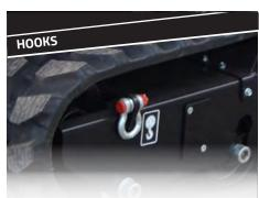
Large and sturdy hooks to move the machine in total safety.
