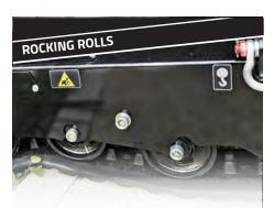
The machine's undercarriage oscillated to follow the terrain pro□le for increased stability and comfort.
